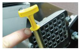
5. After 10 seconds have passed, remove the dip stick.
