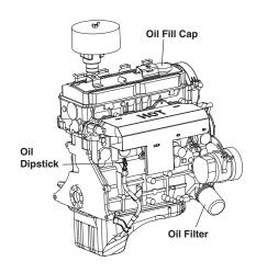
2. The most accurate oil level readings are measured when the engine is cold. If the engine was running, wait at least 10 minutes before proceeding to the next step.
