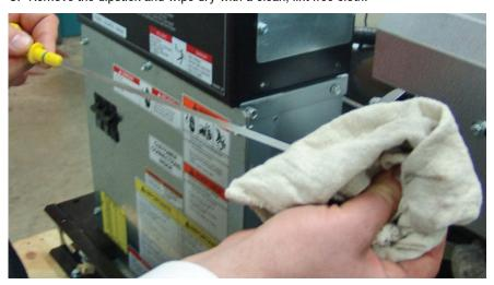
4. The clean dip stick should be **slowly** inserted into the dip stick tube. Visually confirm that the dip stick is fully seated in the dip stick tube. A visual inspection is required because some dip sticks will require more effort than others to fully seat.
